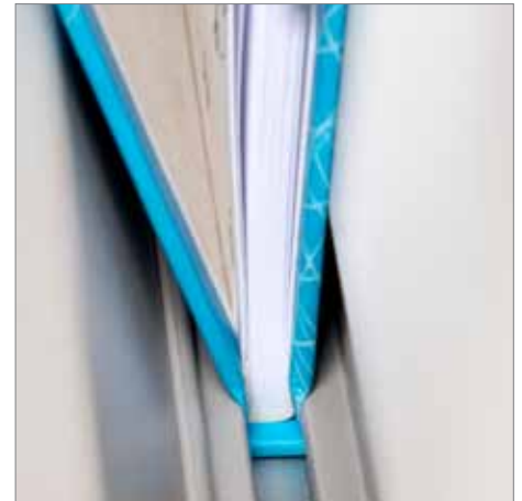
Hot knife groove pressing from two sides simultaneously
